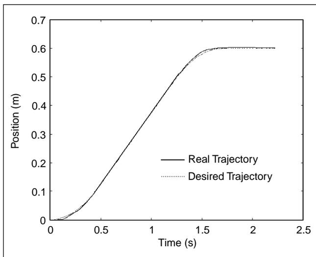
Figure 5. X-axis trajectory (displacement 0.6 m, velocity 0.5 m/s).
