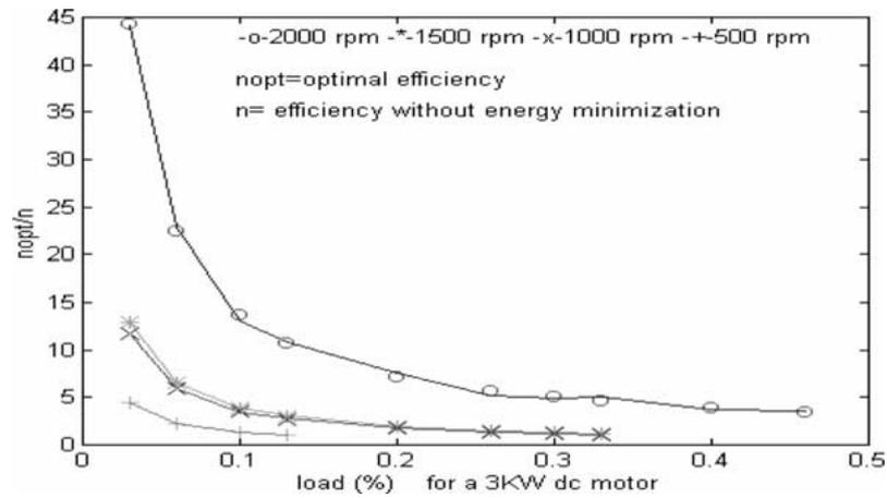
Figure 4. Experimental study for a 3 kW robot dc motor drive: 2%–8% efficiency improvement by the proposed control scheme “Test1” compared with the control scheme “Test2”.
