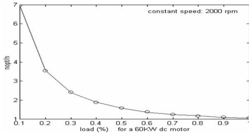
Figure 5. Experimental study for a 60 kW robot dc motor drive: 2%–8% efficiency improvement by the proposed control scheme “Test1” compared with the control scheme “Test2”.
