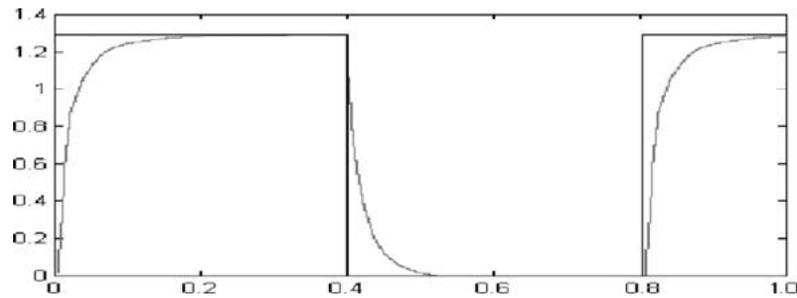
Figure 1. Robot dc motor speed response as derived by the proposed control scheme “Test 1” (Speed control with simultaneous electromechanical losses minimization).
