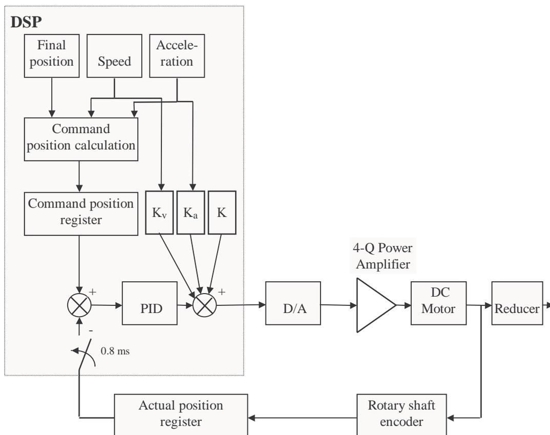
**Fig. 3.** The servo control of each robot axis
