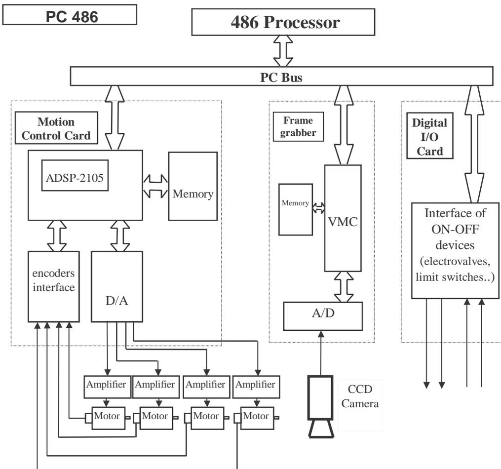
Fig. 2. The overall control scheme
