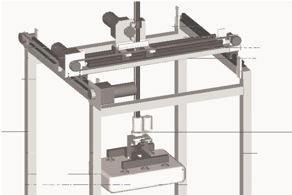
**Fig.1.** The *X-Y-Z-R* Cartesian robotic system
