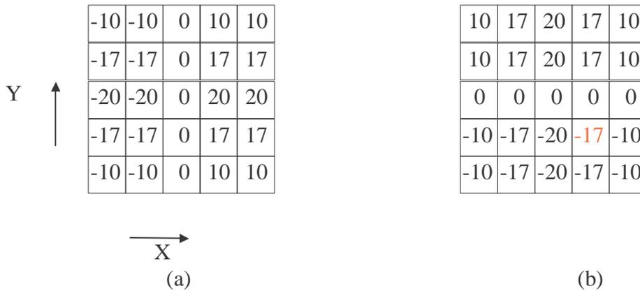
**Fig. 4.** 5x5 Sobel edge detection masks
