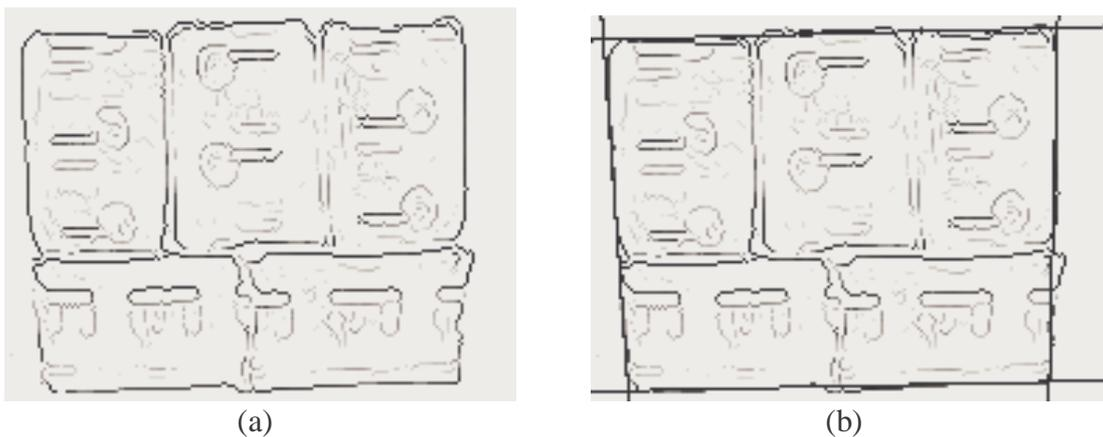
**Fig. 6.** (a) thinned edges, (b) the detected boundary
